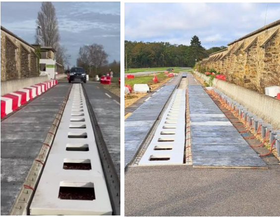
Fig 14 test track in Versailles Satory with Paris coil
