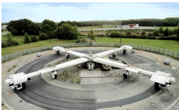
Full scale accelerated pavement testing facility
