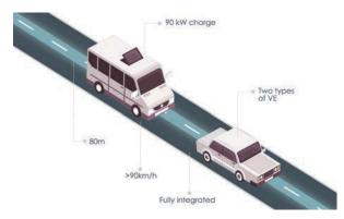
An on-board charger is included in the vehicles to control the charging current. The EV has a lane keeping assistant to improve alignment during charging.
