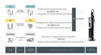
Low cost V2G chargers designed are paralleled to obtain any power rating. In the project, 200 kW super fast chargers have been developed to charge up to 200 km in 10 minutes, whilst providing active and reactive power management in real time to the DSO and TSO, preparing the super-fast charging stations to be manageable by grid operator.
